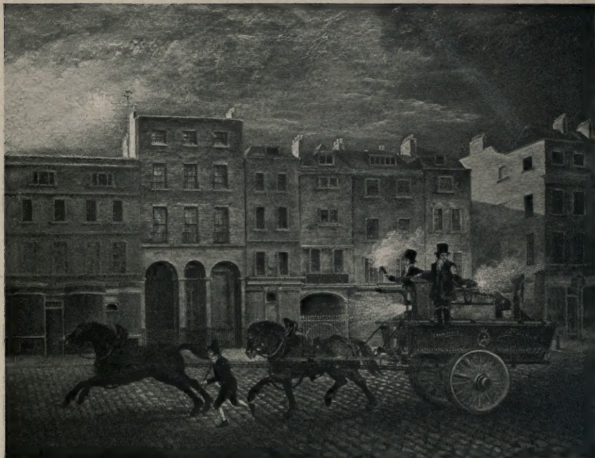
BISHOPSGATE STREET, NR HOUNDSDITCH WITH THE ENGINE AND CART OF THE LONDON ASSURANCE PROCEEDING TO A FIRE. THE LONDON ASSURANCE USED AT THAT TIME A SMALL HAND ENGINE CONVEYED IN A CART MADE FOR THE PURPOSE DRAWN BY TWO OR MORE HORSES TANDEM, THE DRIVER RUNNING BY THE SIDE.
